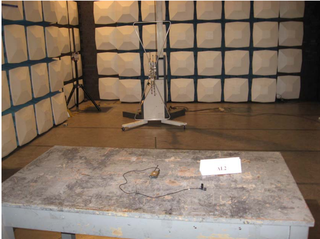
Photograph 1: Set-up for Radiation Measurement below 1GHz
