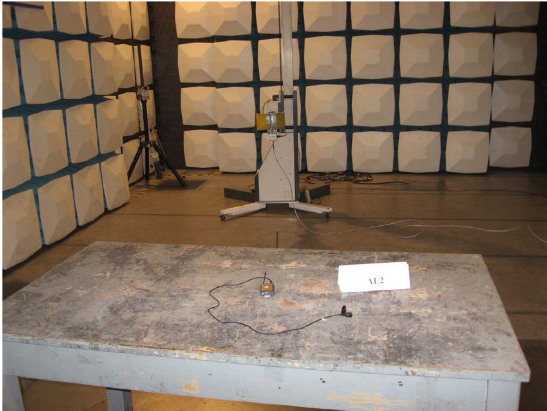
Photograph 2: Set-up for Radiation Measurement above 1GHz
