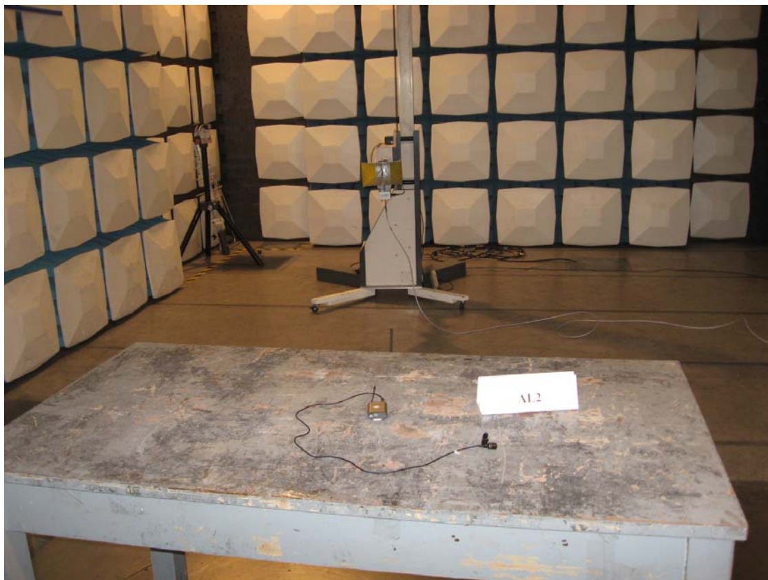
Photograph 2: Set-up for Radiation Measurement above 1GHz
