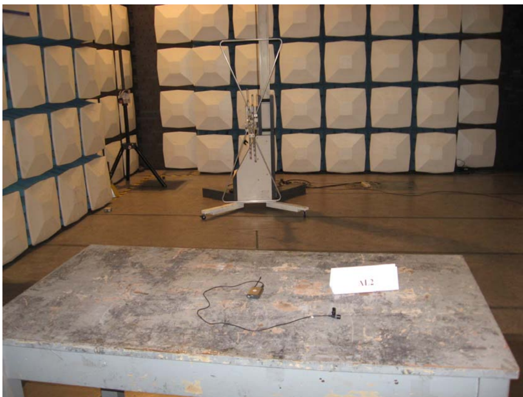
Photograph 1: Set-up for Radiation Measurement below 1GHz
