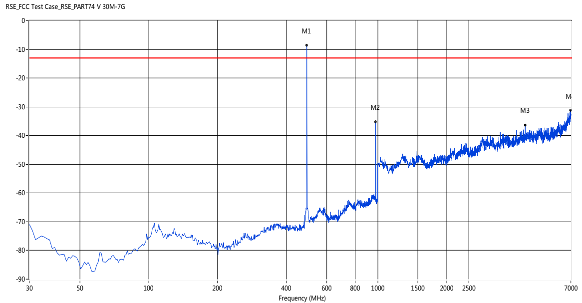
Figure 4: TX Spurious Radiation, 30 – 7000 MHz, Vertical (Middle CH)
