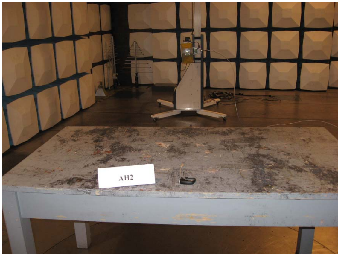
Photograph 2: Set-up for Radiation Measurement above 1GHz
