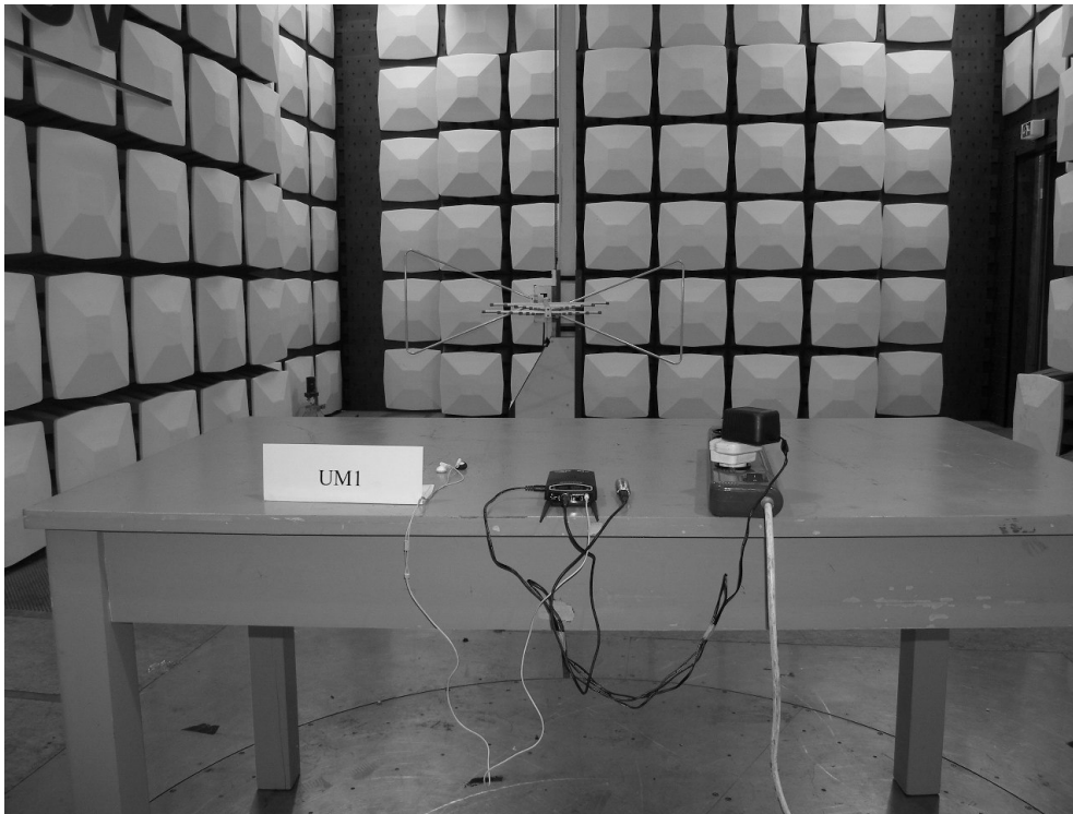
Photograph 2: Set-up for Radiation Measurement below 1GHz
