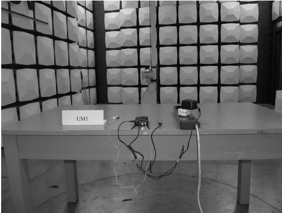
Photograph 3: Set-up for Radiation Measurement above 1GHz
