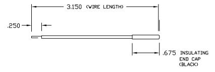
Antenna gain of 1.9 dBi GAnt = EIRP - PTx + LC1.9dBi= 1.3dBm - 23dBm + 23.6
