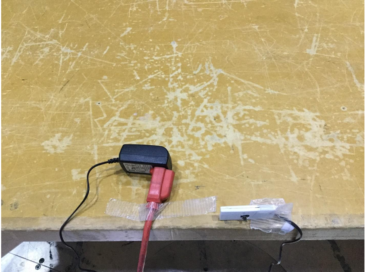
Radiated emissions test setup, 30 MHz – 1 GHz, X-axis
