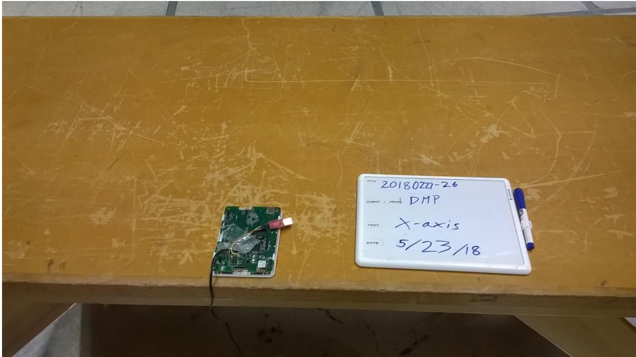
Figure 1 - Test Setup, 30MHz - 1GHz, X axis (testing was performed in all 3 axis for 30MHz – 1GHz measurements)
