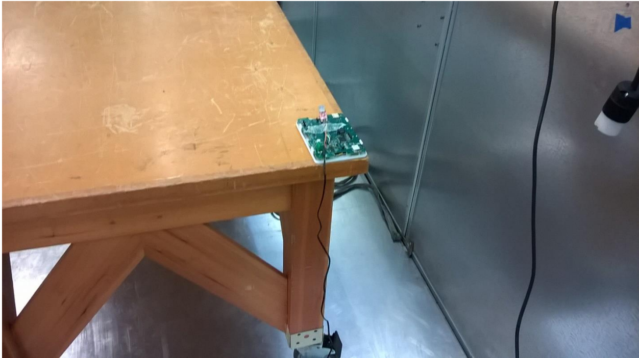
Figure 6 - Conducted Emissions Test Setup
