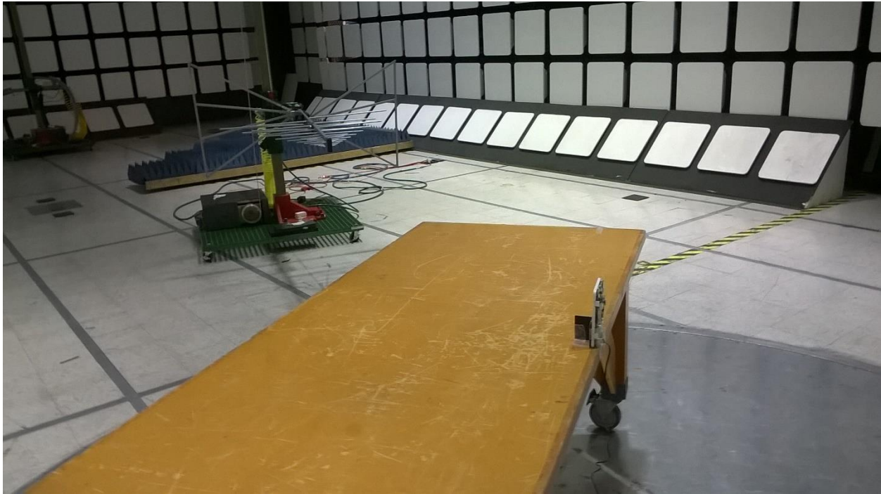
Figure 2 - Test Setup, 30MHz - 1GHz, Z axis (testing was performed in all 3 axis for 30MHz – 1GHz measurements)
