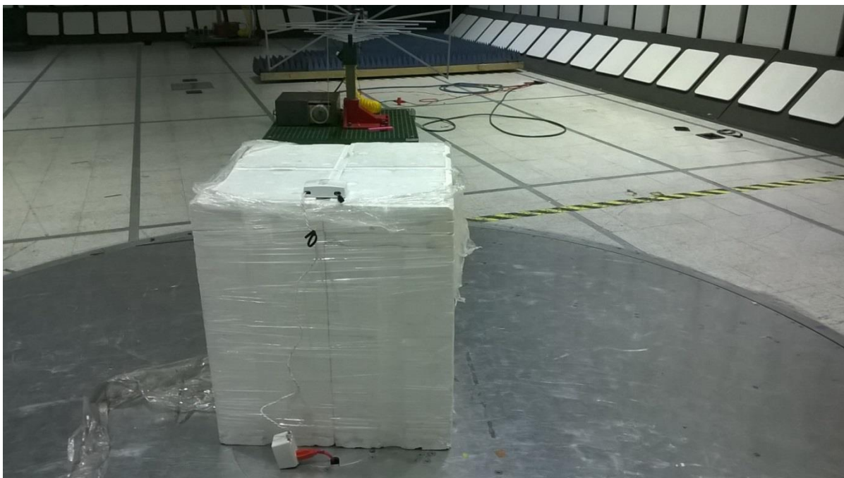
Figure 2 - Test Setup, 30MHz - 1GHz, X axis (testing was performed in all 3 axis for 30MHz – 1GHz measurements)
