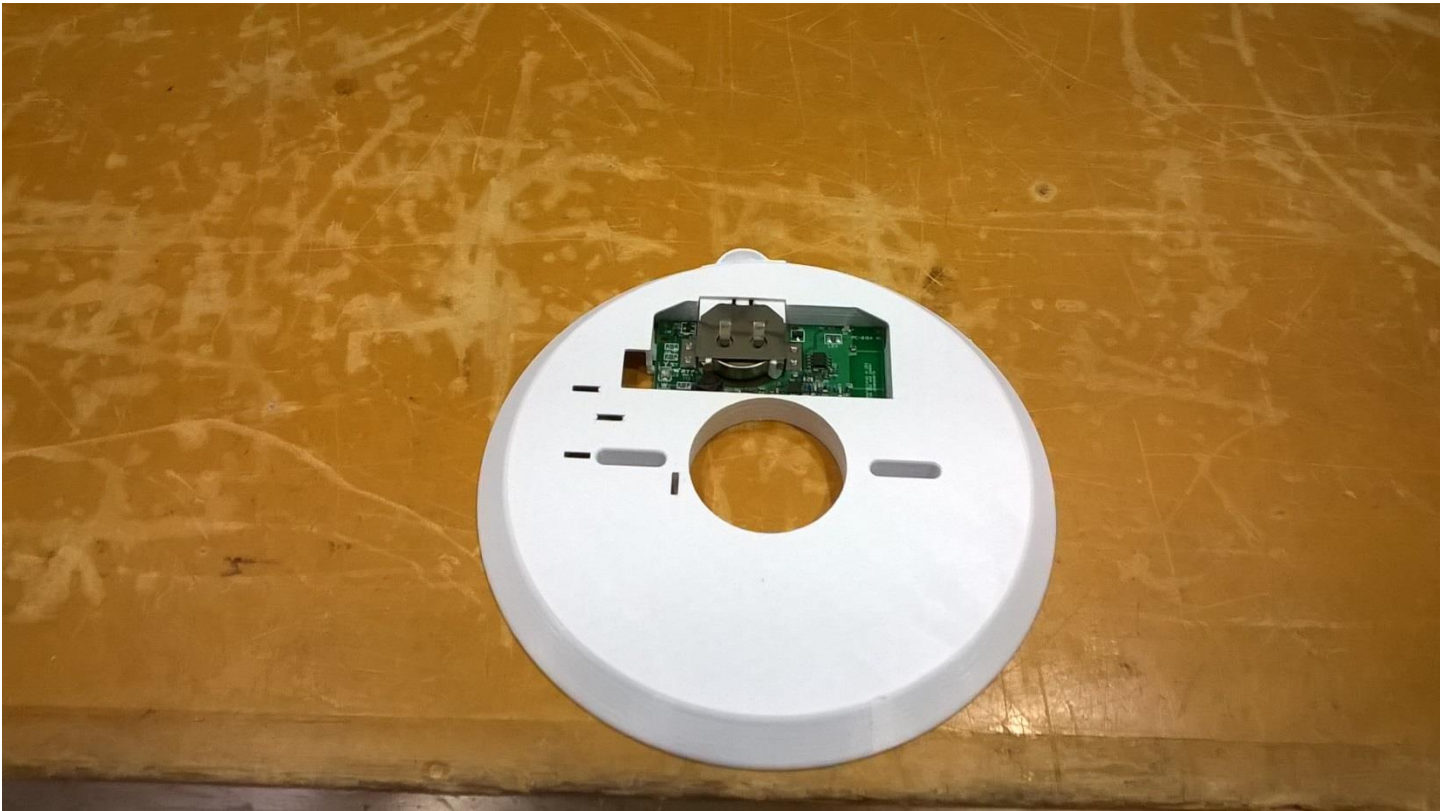
Figure 1 - Radiated emissions test setup, 30MHz - 1GHz, X-axis
