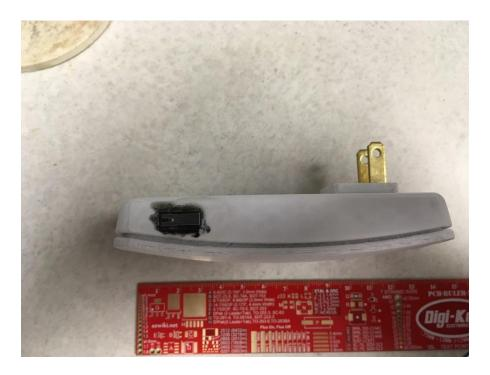
Note: the switch seen on the left side was placed there for testing purposes only. On the standard enclosure there will be nothing there.
