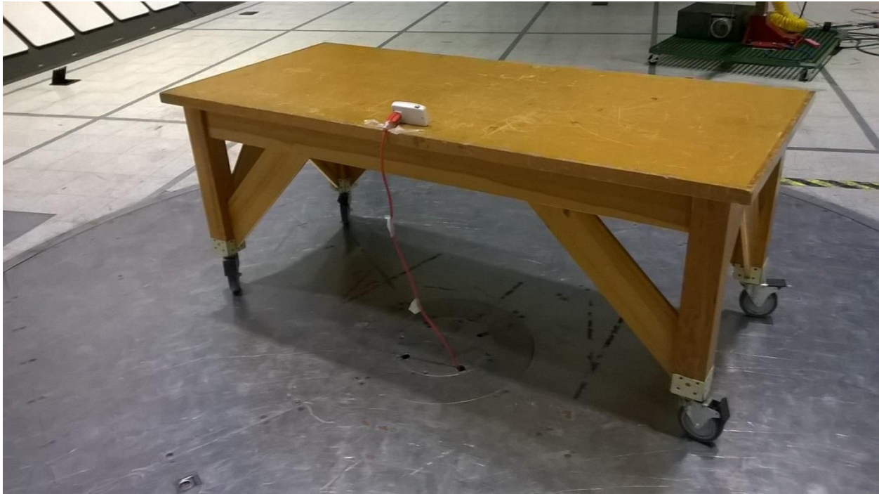
Figure 2 - Test Setup, 30MHz - 1GHz, X axis (testing was performed in all 3 axis for 30MHz – 1GHz measurements)
