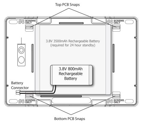
Figure 3: Standby Battery Replacement
