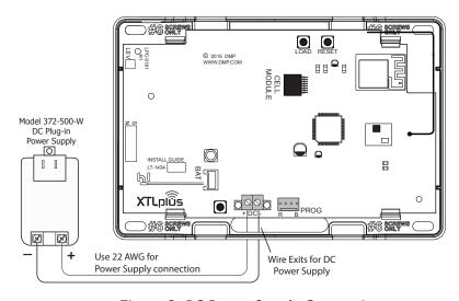
Figure 2: DC Power Supply Connection
