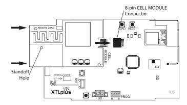
Figure 6: 265C Installed on the XTLplus
