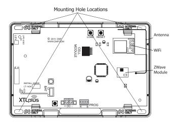
Figure 1: Mounting Hole Locations
