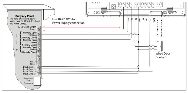
Figure 14: CellComSL Series Wiring Diagram for Zones 1 - 3 and Outputs.
