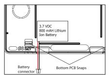
Figure 6: Replacement Battery Locations
