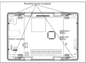
Figure 11: Mounting Screw Locations
