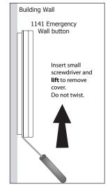
Figure 6: Removing the Cover
