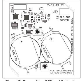
Figure 7: Transmitter PCB and Batteries
