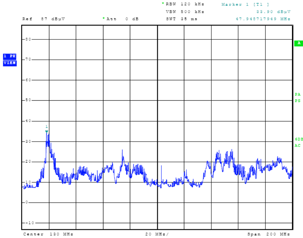
Figure Three General Radiated Emissions taken at 1 meter in screen room
