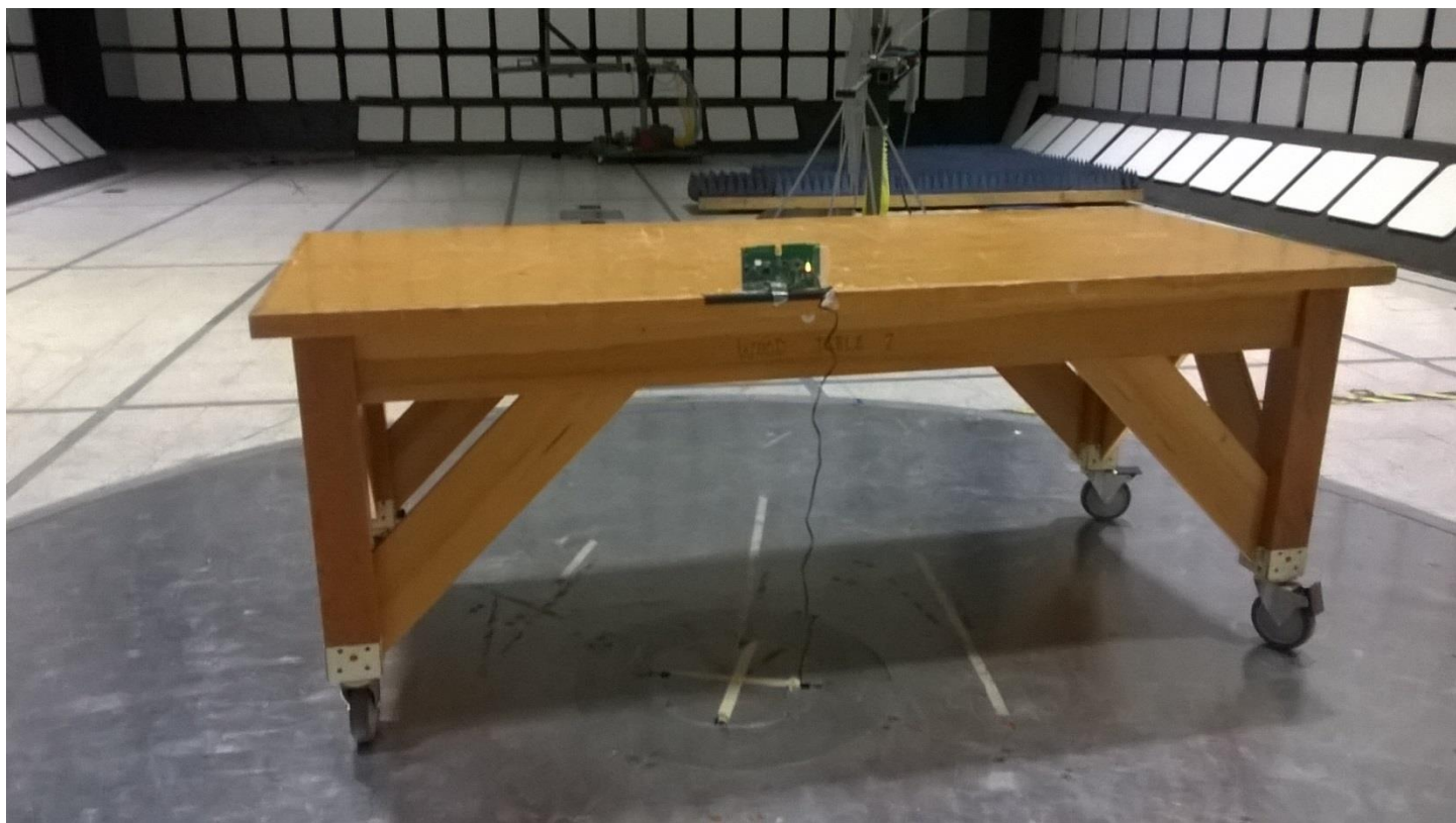
Figure 1 – Radiated Emissions Test Setup, 30MHz – 1GHz
