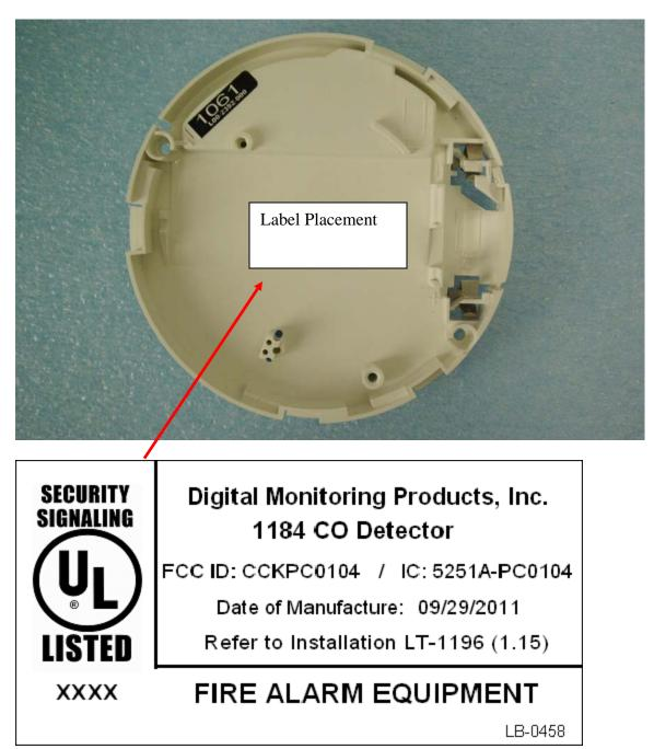
Rogers Labs, Inc. 4405 West 259<sup>th</sup> Terrace Louisburg, KS 66053 Phone/Fax: (913) 837-3214 Revision 1 Digital Monitoring Products, Inc. Model: 1184 CO Detector Test #:110914C SN: W30CO ENG1 Test to: FCC Parts 2 and 15.249, RSS-210 File: LabelSmpl CCKPC0104
