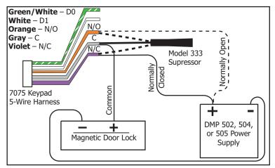
Figure 3: 7075 5-wire Harness and Suppressor Installation
