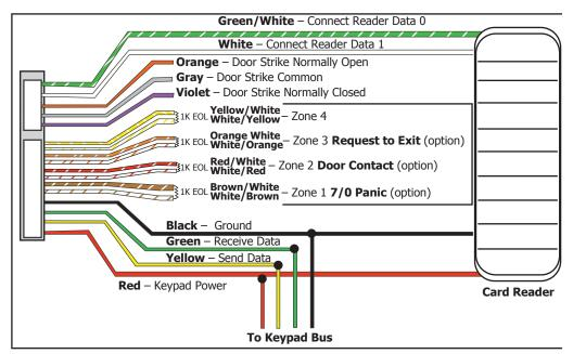
Figure 2: 12 VDC Reader Wiring for 7075 Keypads
