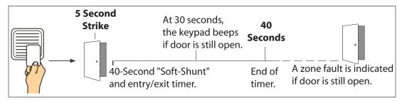
Figure 4: Door Strike Relay Operation Time Line
