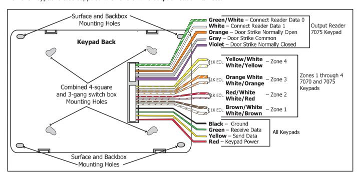
Figure 1: Keypad Back Showing Wiring Harness Assignments
