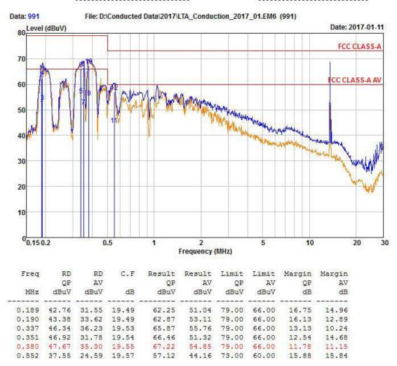
Remarks: C.F (Correction Factor) = Insertion loss + Cable loss + Pulse Limiter
