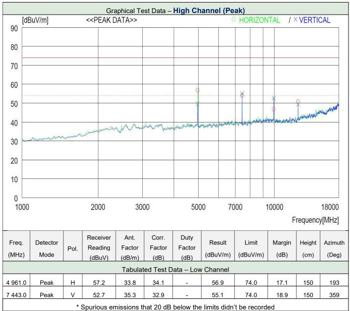
Corr. Factor (dB) = Pre-amplifier gain - Cable Loss
