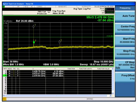
Conducted Spurious Emissions 3 (Test Channel : 2440 MHz)
