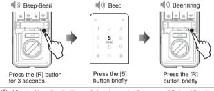
(i) After double authentication mode is set up, enter the password first and then touch
