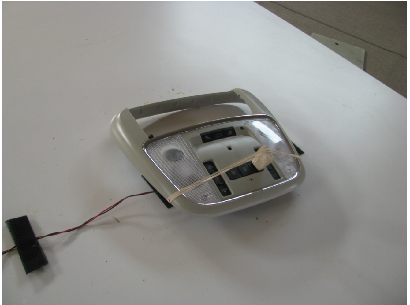
Test Setup Photograph 3: Device Tested lying flat. The button was depressed for constant transmit using a block and elastic band.
