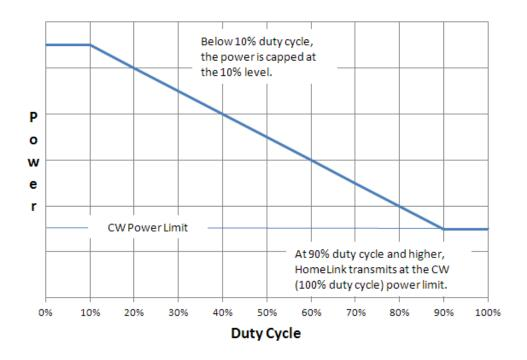
To verify correct operation, I trained the HomeLink module to signals with different duty cycles and measured the output power. I verified that 90% and 95% duty cycles had essentially the same output power, while the power increases for lower duty cycles. Since HomeLink is unable to train to a 100% duty cycle signal, I was unable to include that in the testing.
