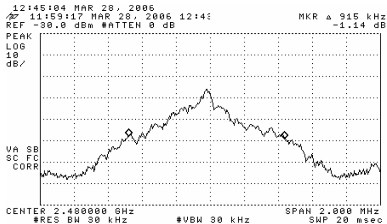
Figure 6.1 Measurement of channel 20 dB bandwidth. (top) Low Channel, (middle) Middle Channel, (bottom) High Channel
