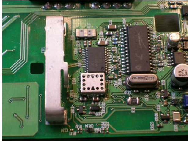
Figure 8.4.1 Close-up of Homelink RF Section.
