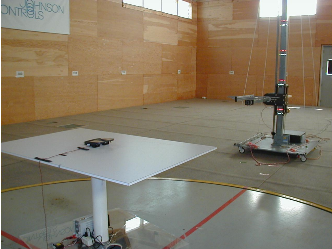
Figure 3.1 The JCI 3m Radiated Emissions Test Setup.
