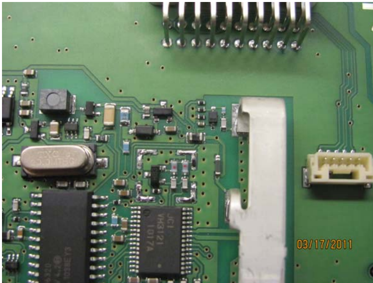
Close-up of Homelink RF shield removed
