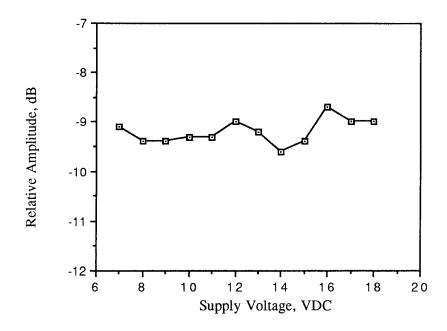
Figure 6.4. Relative emission vs. supply voltage. (310 MHz, continuous pulsed, 50% duty)
