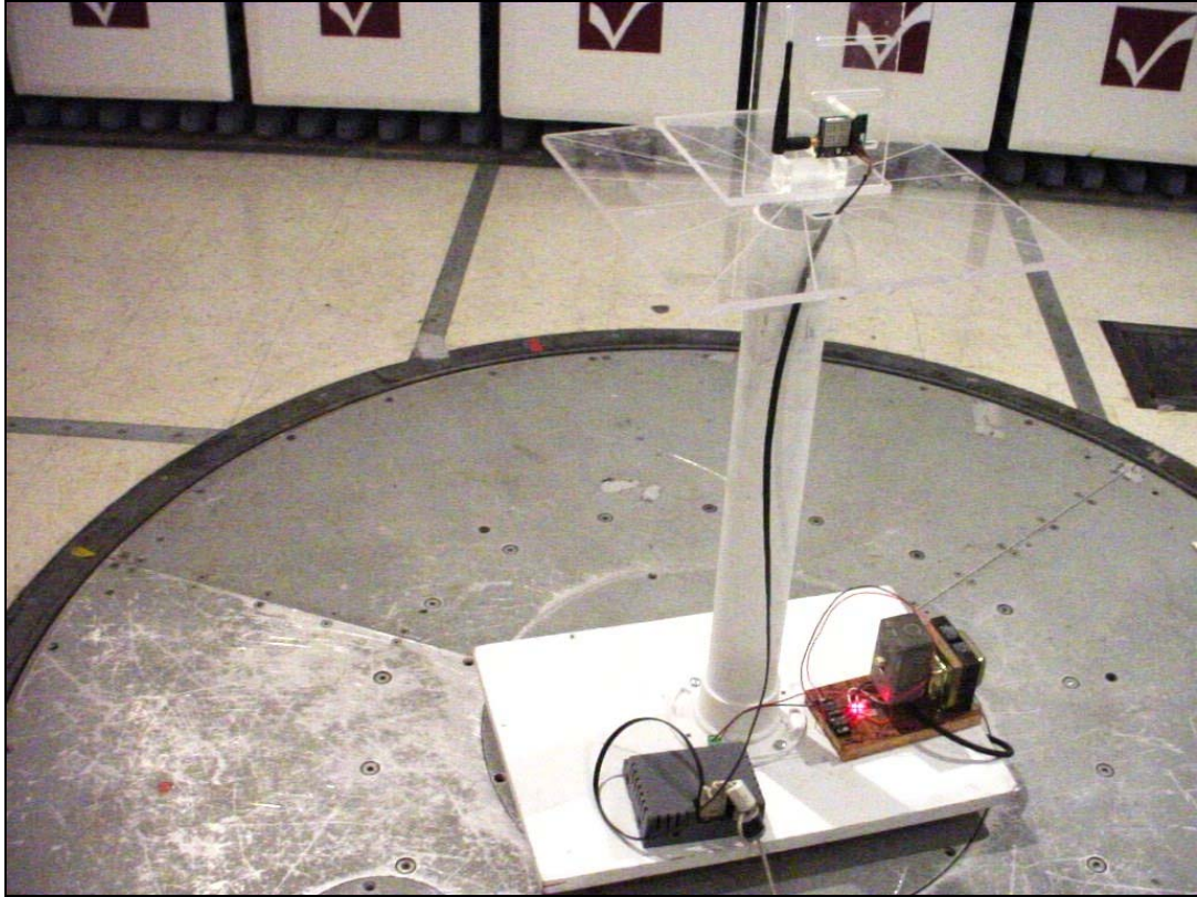
General setup of the EUT on the test stand during radiated emissions tests.
