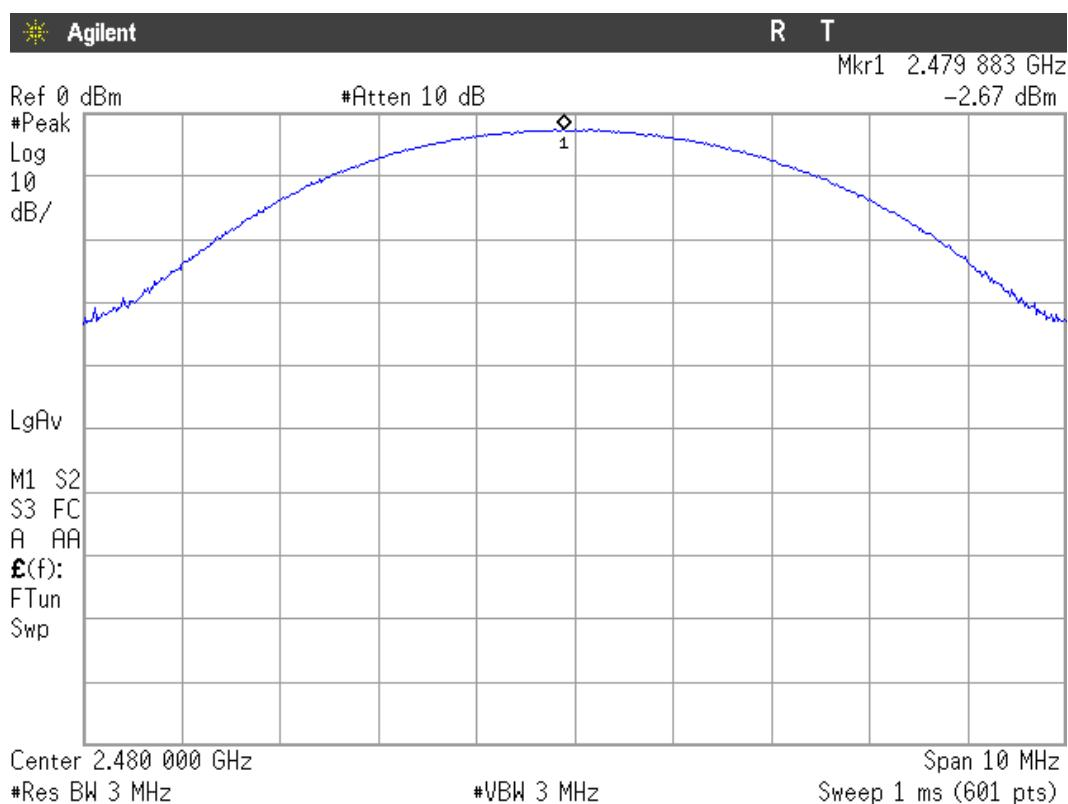
**FCC Section 15.247 Subclause (d) / RSS-210 Clauses 2.2 & A8.5. Band-edge compliance of conducted emissions (Transmitter)**
