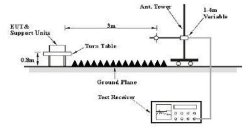
The radiated emission were performed in the 3 meters chamber test site, using the setup accordance with the ANSI C63.4-2014. The specification used was the FCC Part 15.109 and ICES-003 Class B limits.
