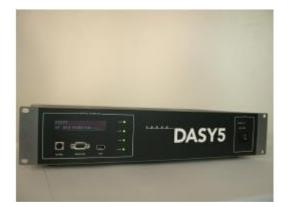
The measurement server performs all real-time data evaluation of field measurements and surface detection, controls robot movements and handles safety operation. The PC operating system cannot interfere with these time critical
