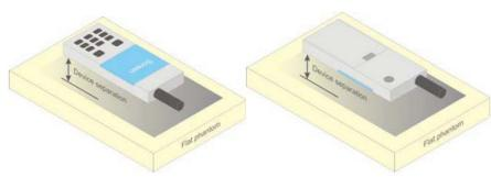
Figure 5 – Test positions for body-worn devices
