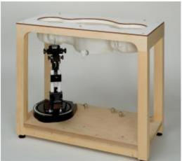
standard measurement positions in the three sections. Only one device holder is necessary if two phantoms are used (e.g., for different liquids)
