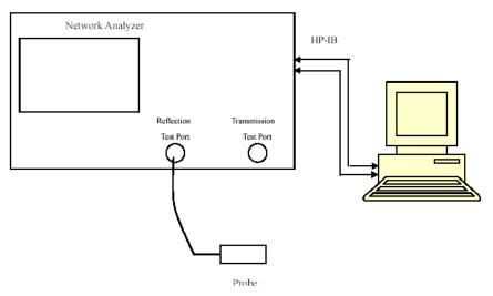
Liquid Verification Setup Block Diagram
