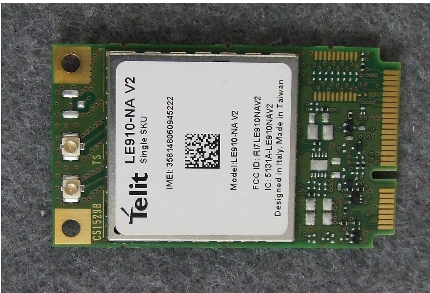
Photograph 13: Front Cellular Module
