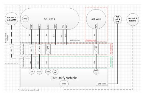
In the above diagram "ANT unit 1" is a multi-bearer "Sharkee" antenna (GPSD-7-27-24-58-T), produced by Panorama antennas which has a gain of 4dBi. "ANT unit 2" is a PCTEL WLP2458NGP-T that has a gain of 3.9dB in the 2.4GHz band and 3.0dBi in the 5GHz band.
