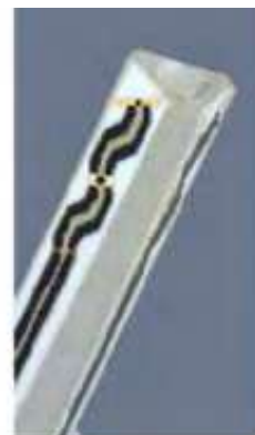
Figure 2.3 Probe Thick-Film Technique
