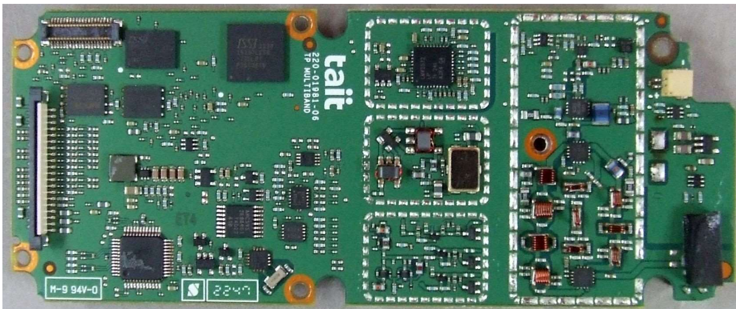
Photograph 02: Receive-Transmit PCB - top (without shields)
