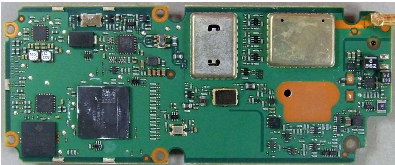
Photograph 03: Receive-Transmit PCB - bottom (with shields)
