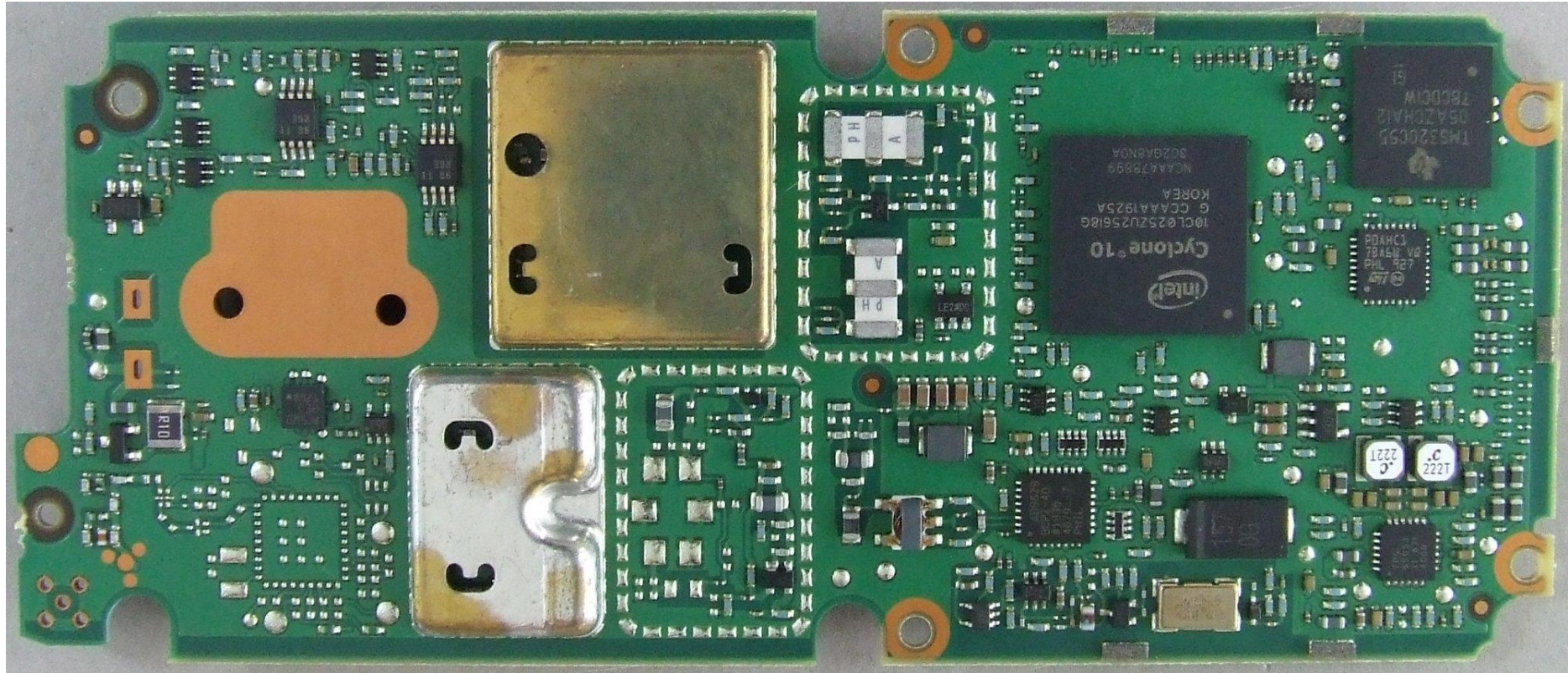
Photograph 03: Receive-Transmit PCB - bottom (with shields)
