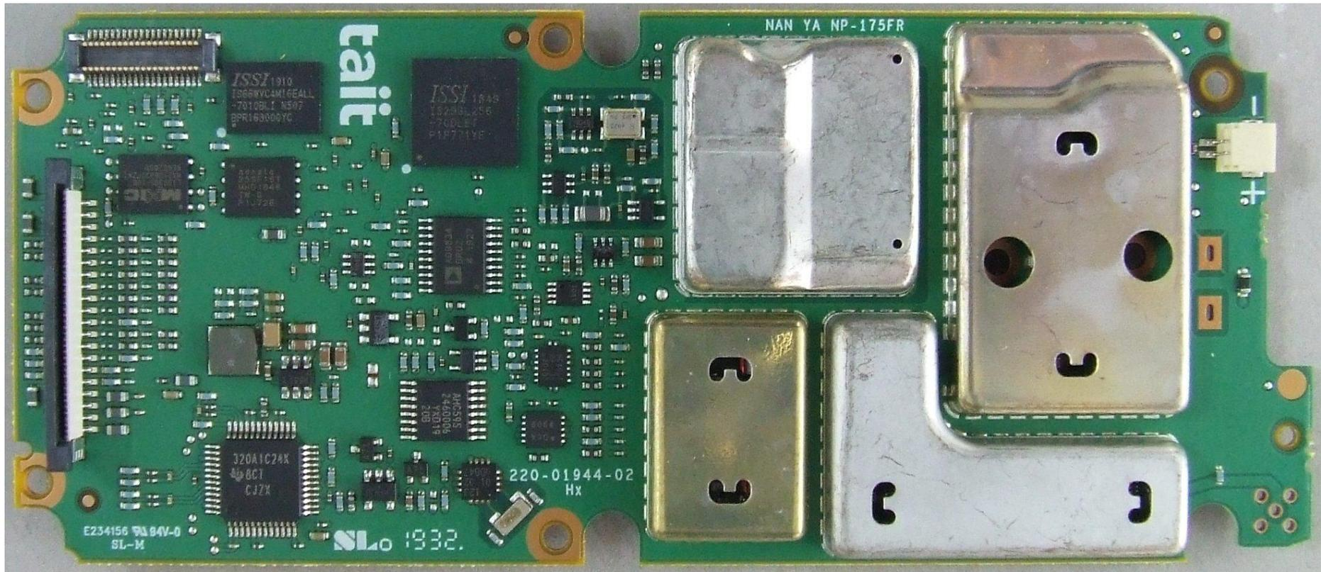
Photograph 01: Receive-Transmit PCB – top (with shields)
