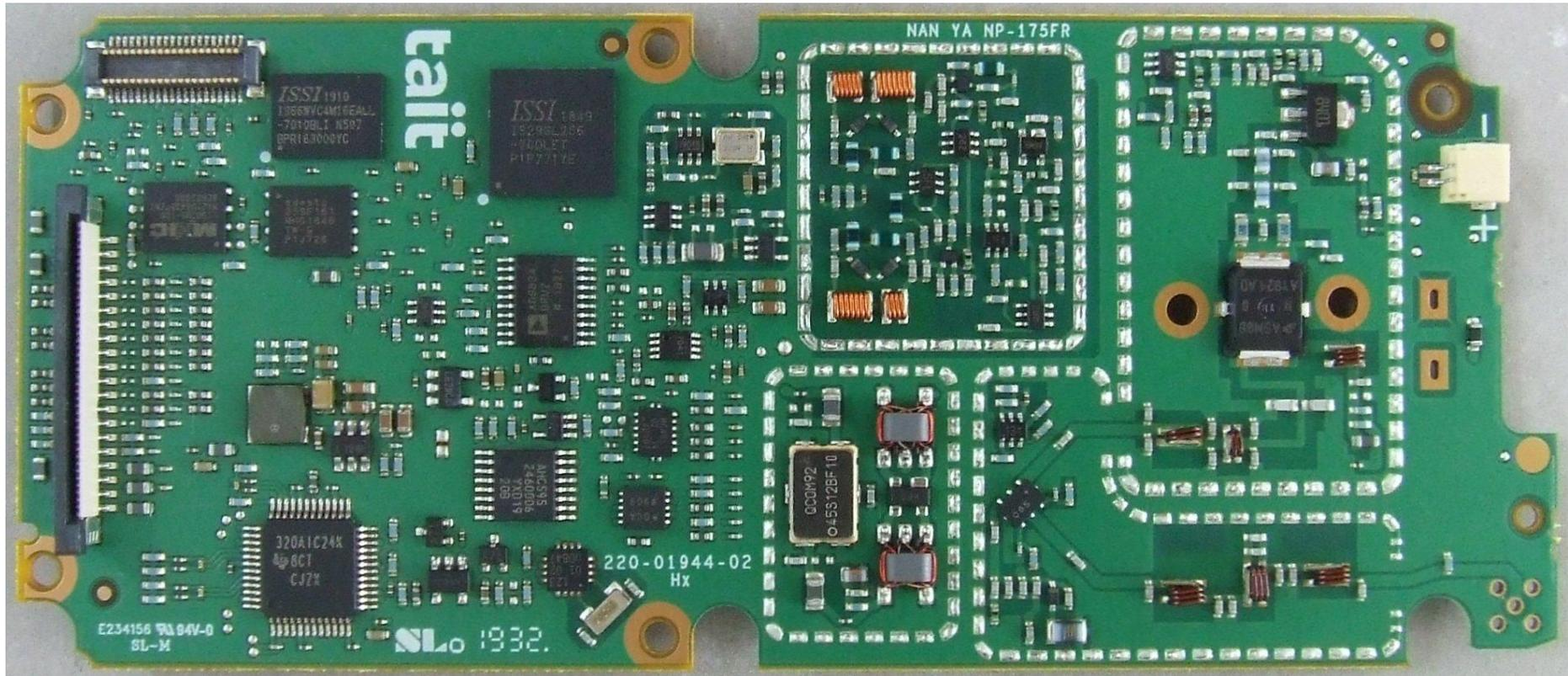
Photograph 02: Receive-Transmit PCB - top (without shields)
