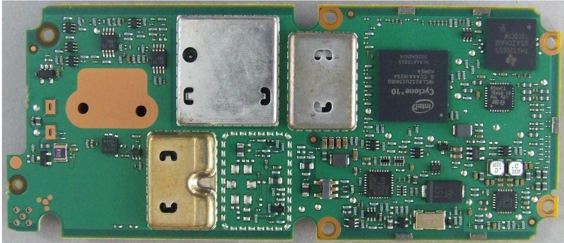
Photograph 03: Receive-Transmit PCB - bottom (with shields)
