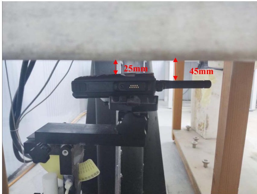
Face Up Setup Photo (25mm)( Short antenna)
