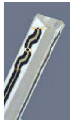
Figure 2.3 Probe Thick-Film Technique
