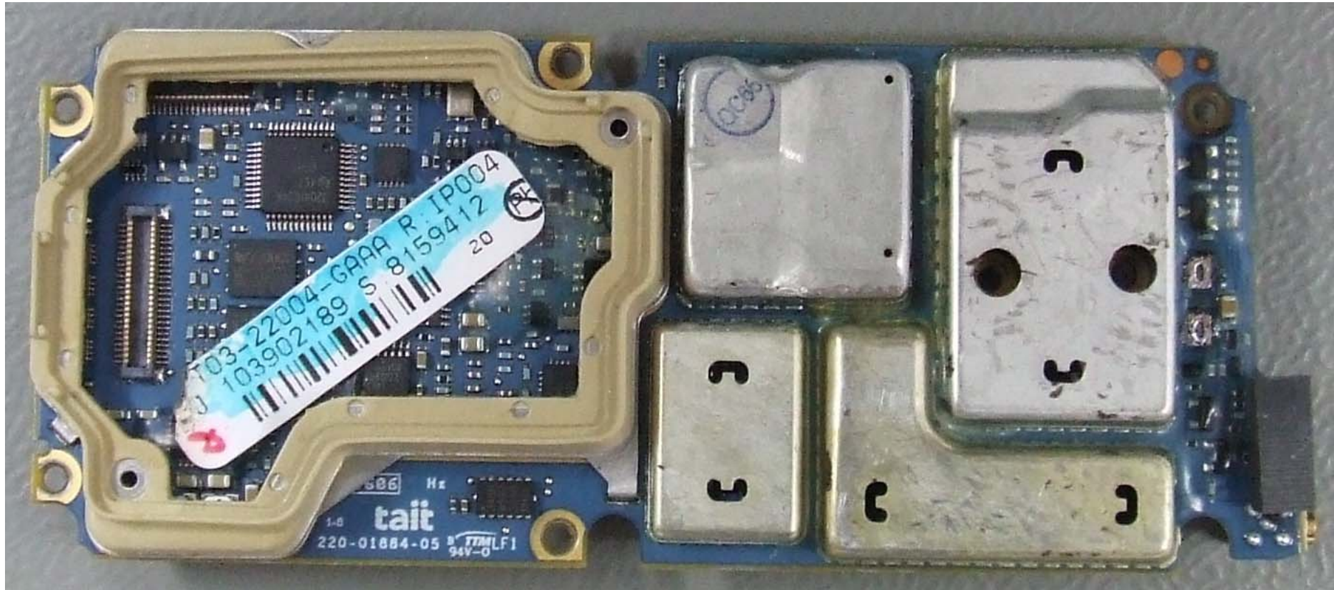
Photograph 02: Rx-Tx PCB - top (with shields)
