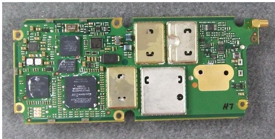
Photograph 04: Rx-Tx PCB - bottom (with shields)
