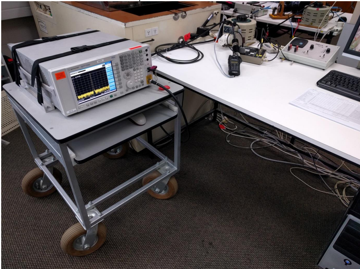
Photo: Conducted Emissions Test Setup
