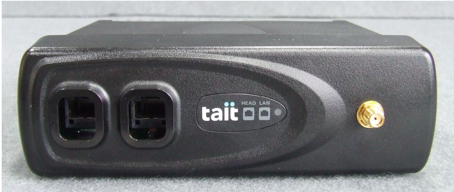
Photograph 03: UnifyVehicle attached to Mobile Radio – front
