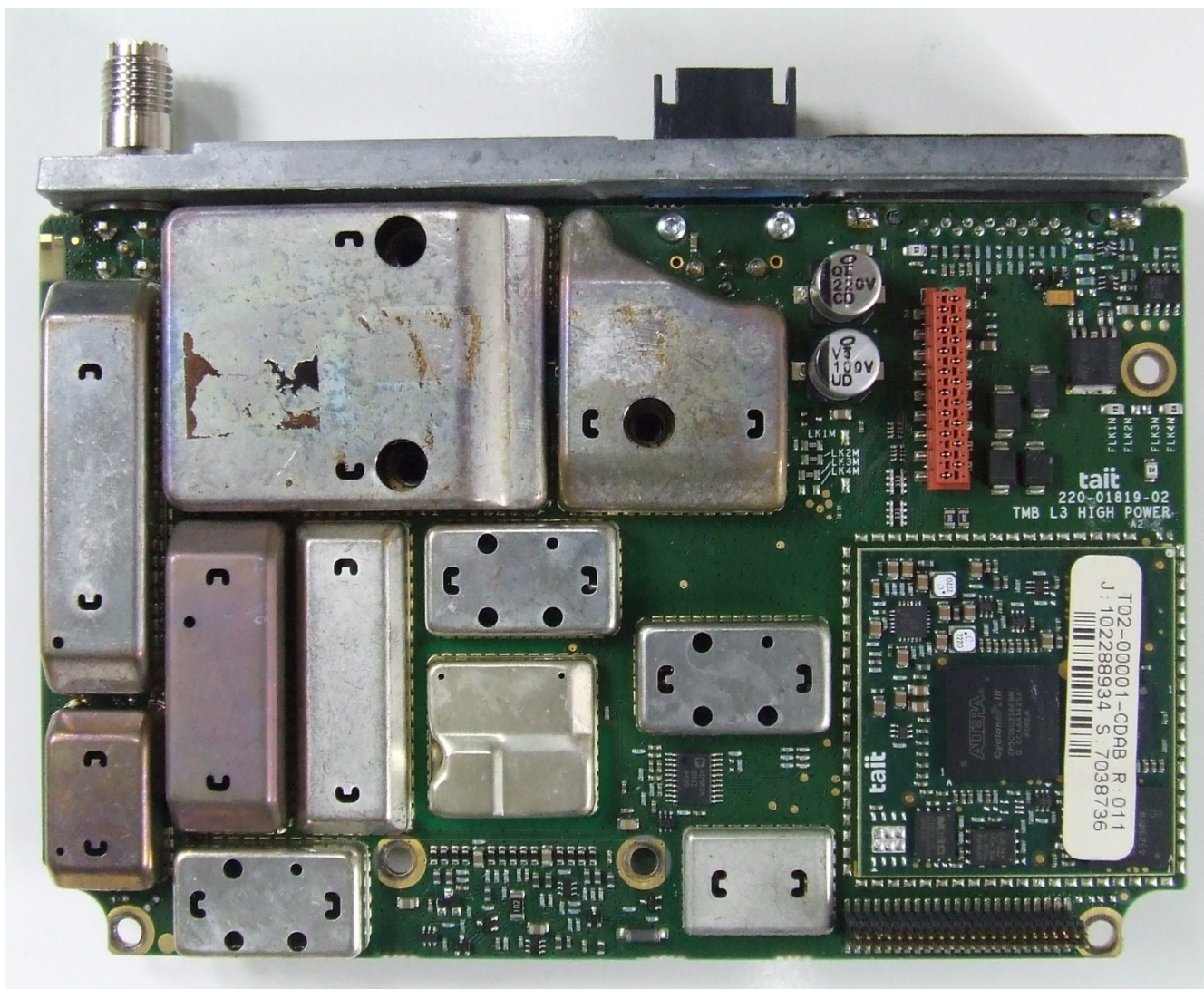
Photograph 01: Radio - Main PCB top with shields
