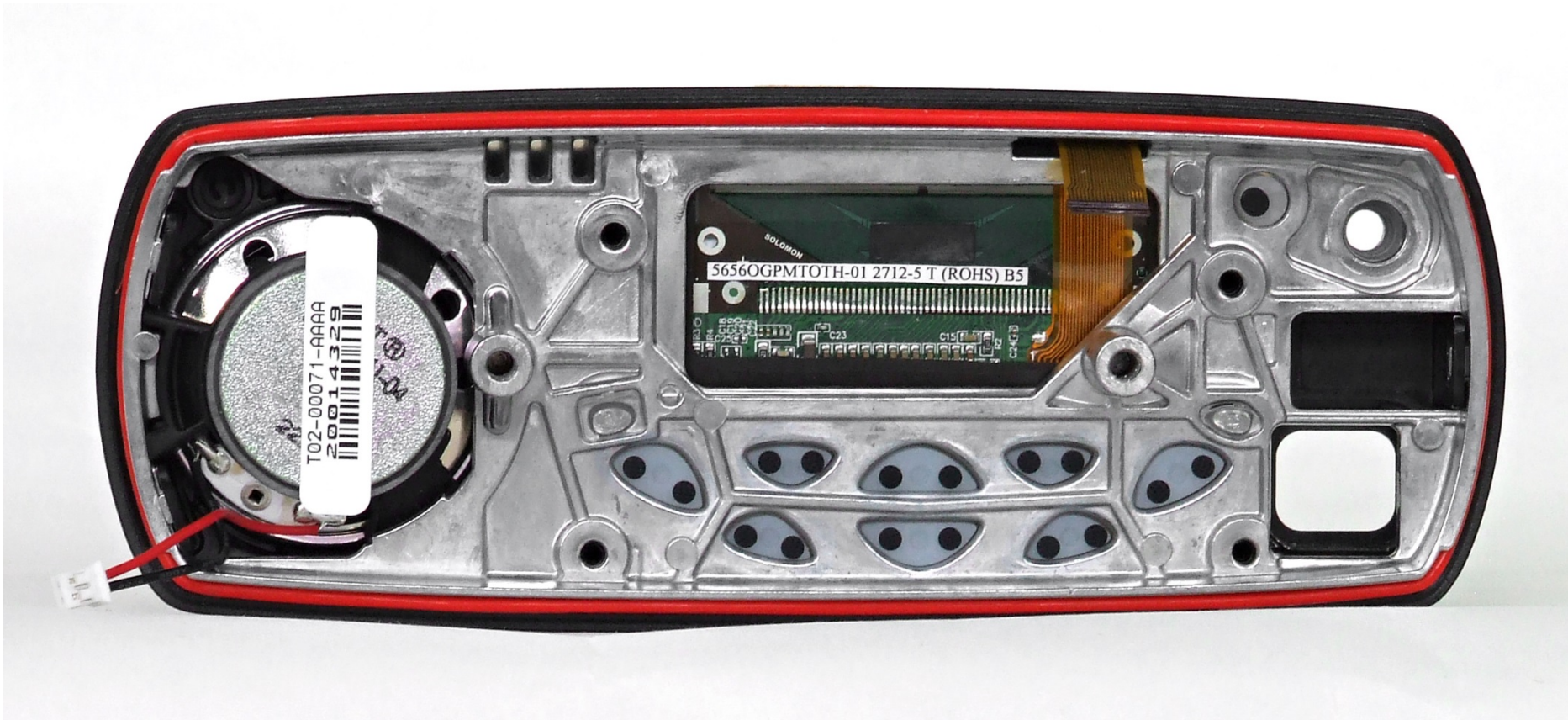
Photograph 06: Control Head – Internal with main PCB removed
