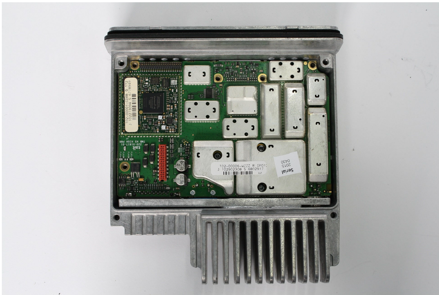
Photograph 03: Radio - Main PCB top with shields inside torso
