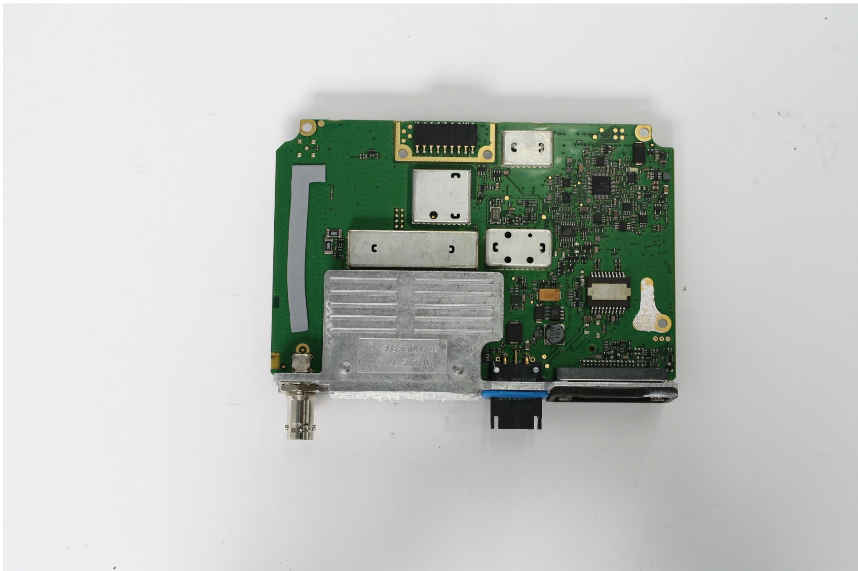
Photograph 05: Radio - Main PCB bottom with shields
