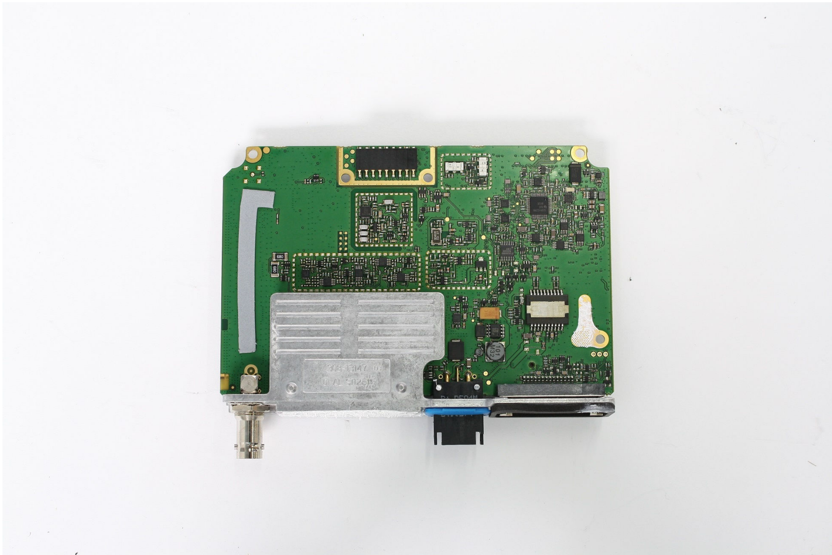
Photograph 06: Radio - Main PCB bottom without shields
