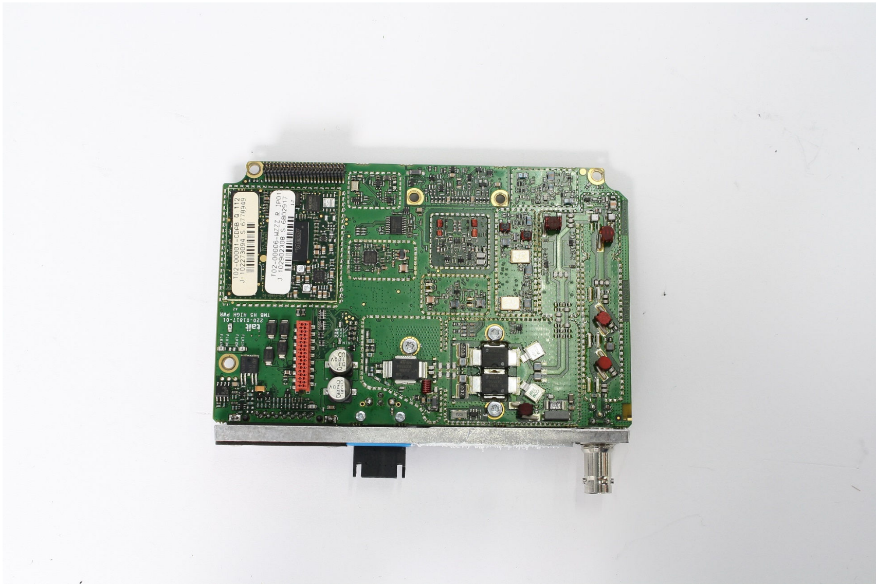
Photograph 04: Radio - Main PCB top without shields
