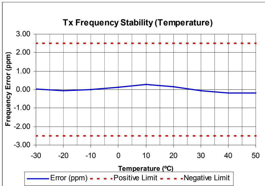
Tx FREQUENCY: 425.1 MHz 40 W 25.0 kHz channel Spacing
